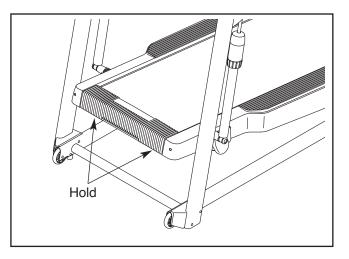
To increase the incline, raise the frame until you hear a click. To decrease the incline, raise the frame until you hear a click and then lower the frame. Make sure the frame is locked securely at one of the incline levels.
